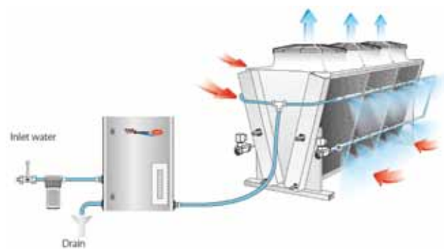
Fig. 3 Schematic for the ChillBooster™ showing how the high ambient temperature air is cooled by water droplets before passing over the coil.
